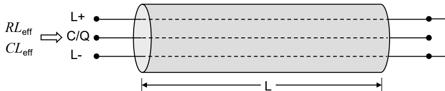
866 Figure 27 – Reference schematic for effective line capacitance and loop resistance
