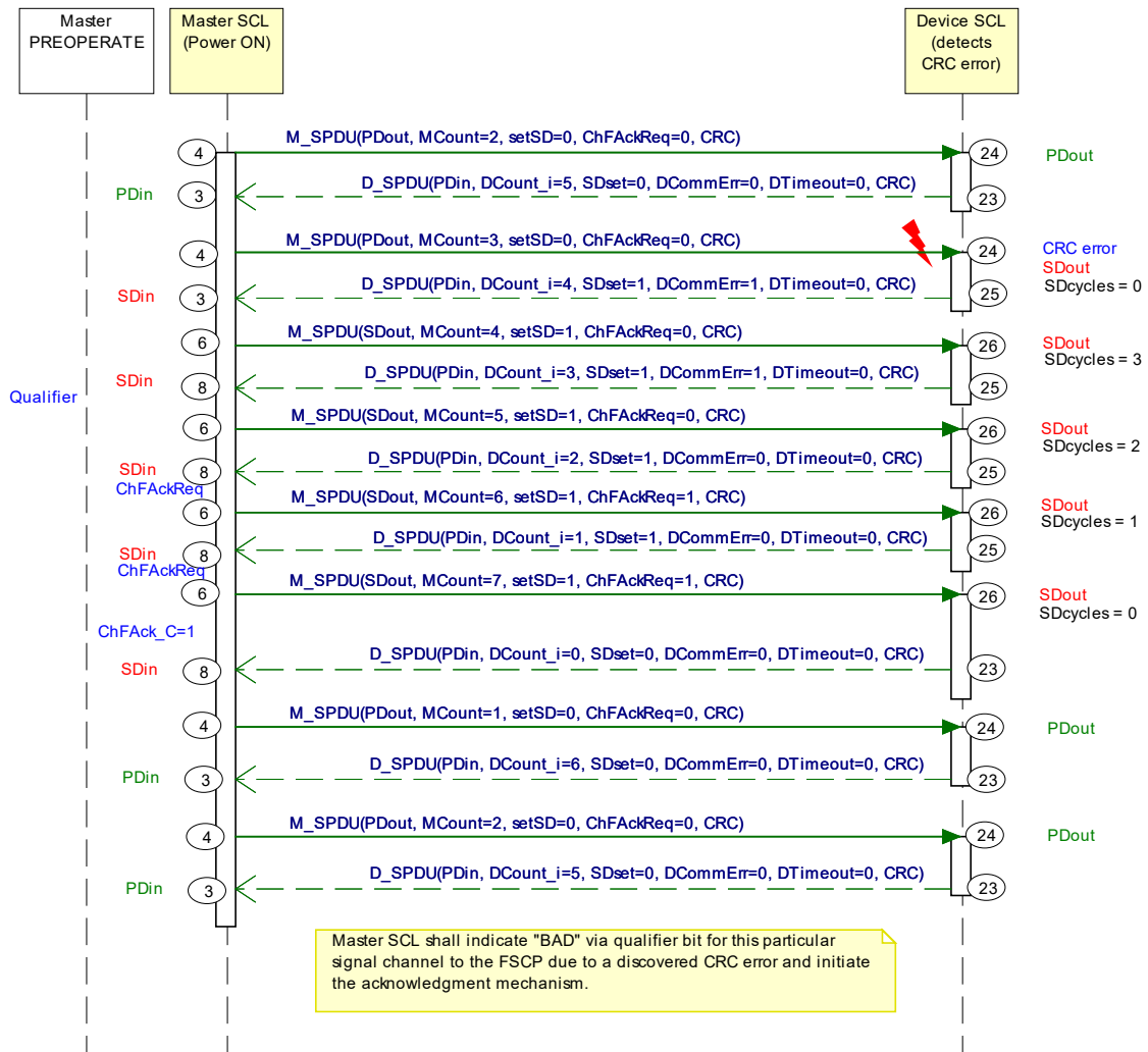
1964 Figure 52 – FS-Device detects CRC signature error
